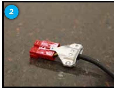
Anderson connector located on charger cable
