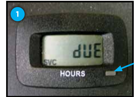
Hour meter showing "SVC DUE"
