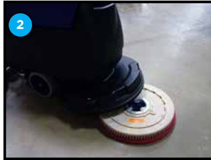
Position scrub head over pad driver(s) or brush(es) (S-20 shown)
