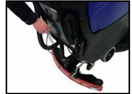
Lowering the squeegee assembly
