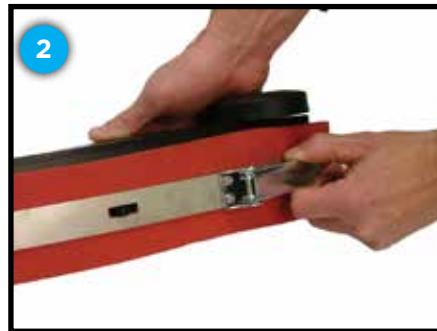
To flip or replace squeegee blades, release over-center latch
