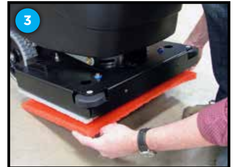
For pad removal on the orbital unit, simply pull off the pad
